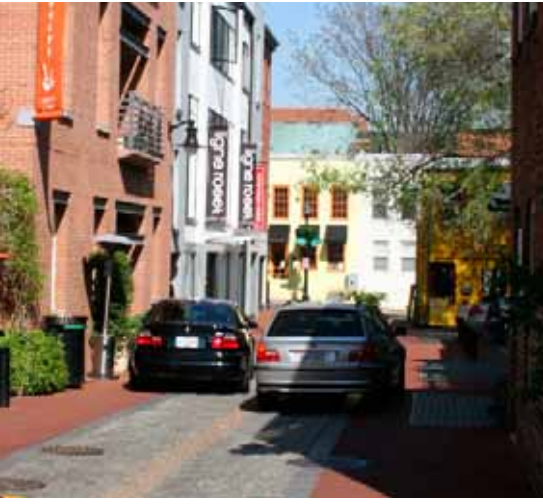
FIGURE 3.31 Private Alley: Two-Way with Bollards and No Curb
