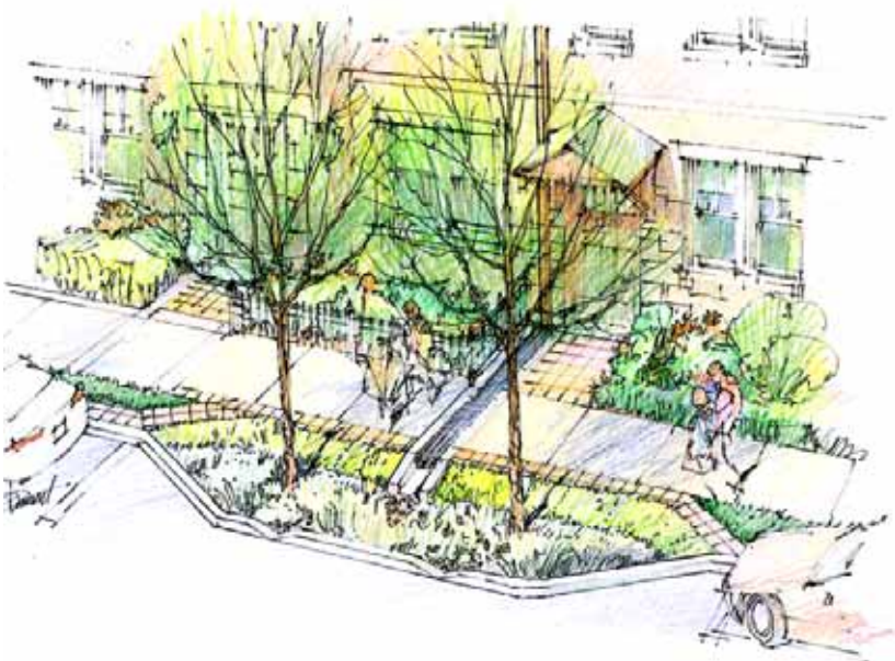
FIGURE 1.10 Precedent sketch showing roof runoff channeled to bioswales in curb bumpout planters
