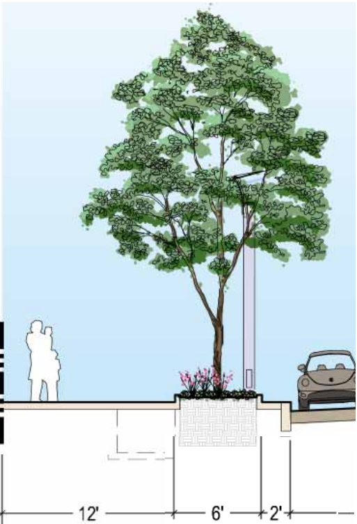
FIGURE 3.28 Sidewalk Type C Section
