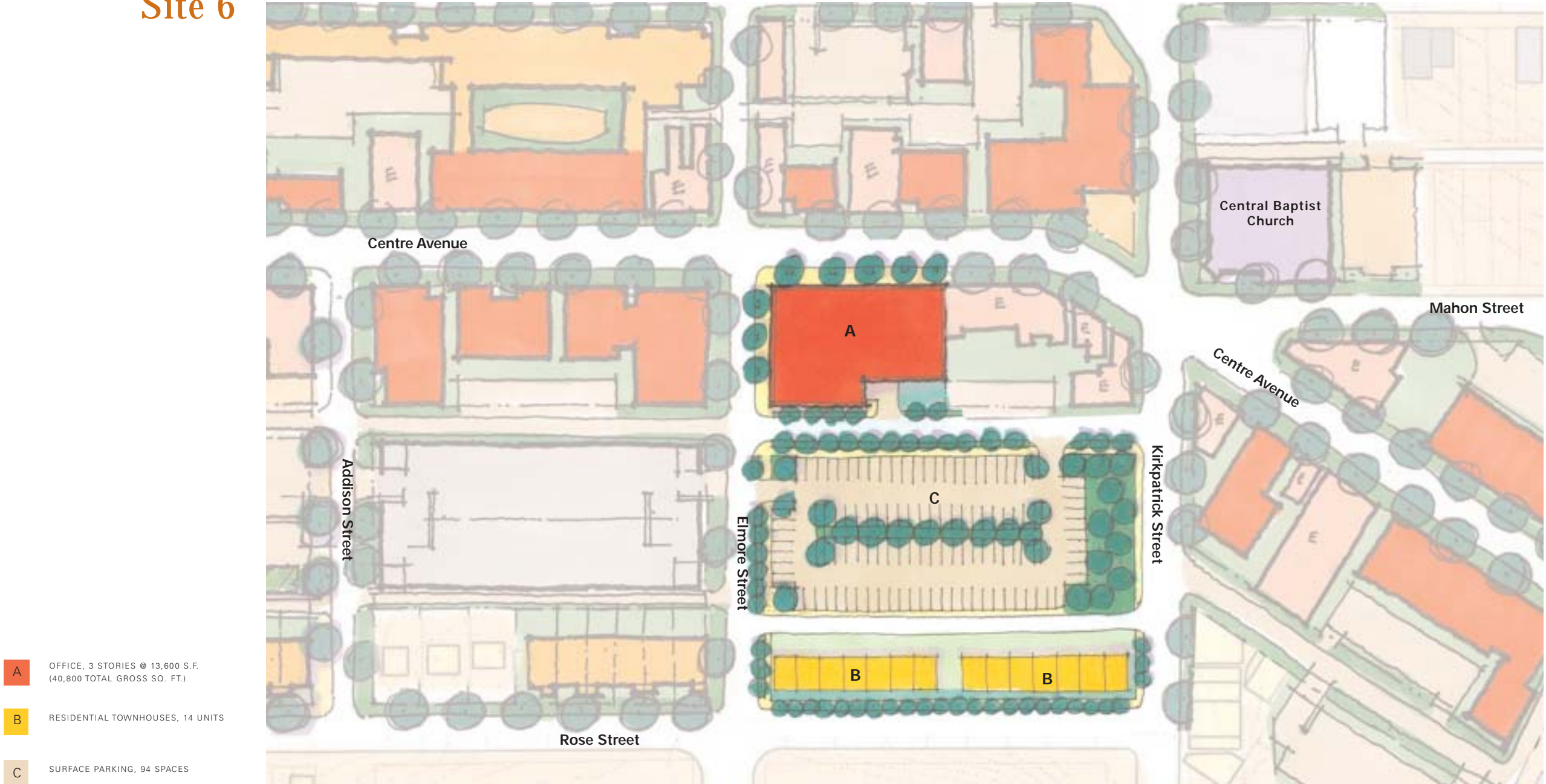
Site 6 contains the 50,000-square-foot Urban League office building on the corner of Centre and Elmore . Surface parking located behind it. The parking lot's edge along Kirkpatrick is buffered with a large, landscaped green. A row of townhouses is proposed on Rose Street to reinforce the residential fabric to the south.
