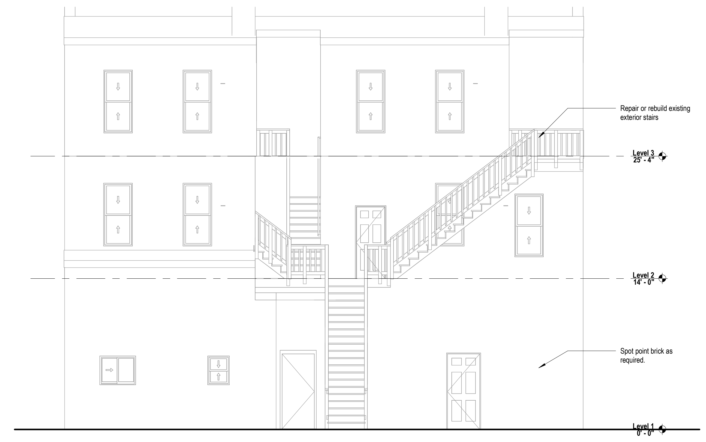
4 North Building Elevation 3/16" = 1'-0"
