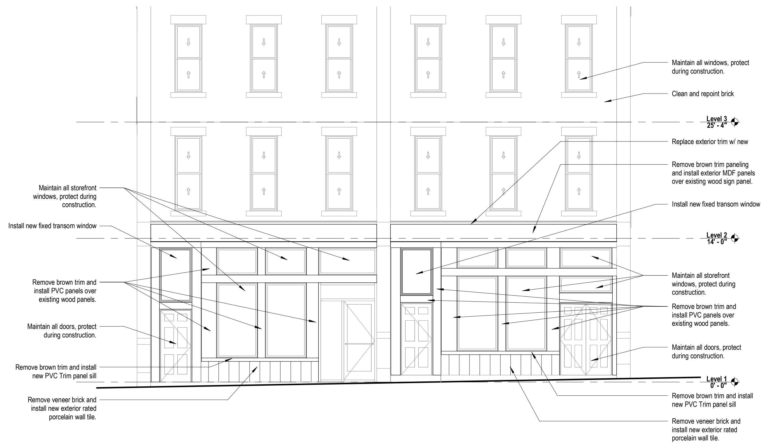
3 South Building Elevation 3/16" = 1'-0"
